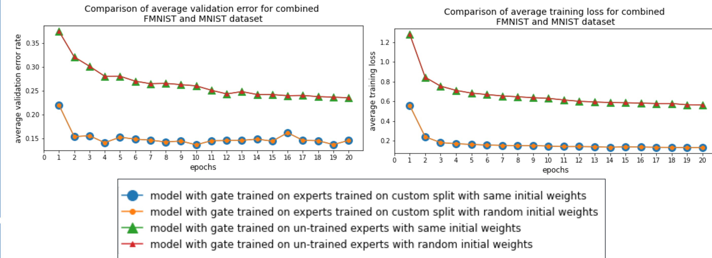
Figure 4 Comparison of training loss and validation error for pre-trained gate, trained with experts pre-trained on custom partition of classes and un-trained experts, and then training new experts with default parameter initialization and experts with the same initial parameter initialization as the experts trained from for MNIST and combined FMNIST and MNIST datasets.
